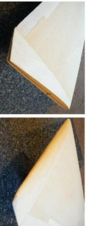
Draw a line along the wing tip then sand to shape
